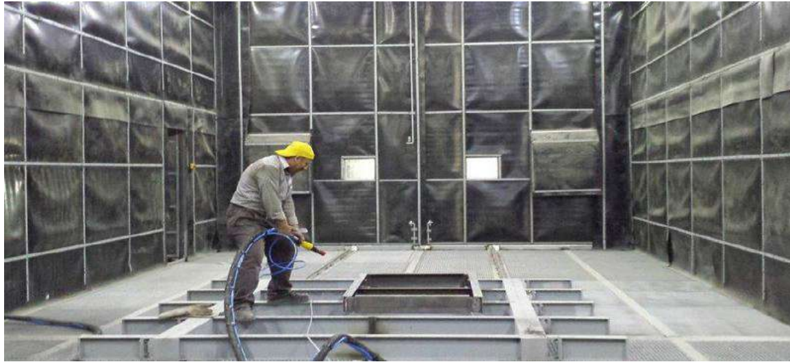
Manual blasting chambers
